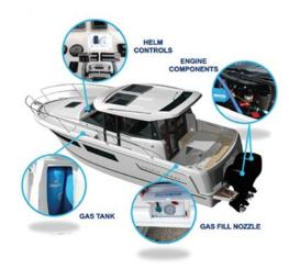
Figure 3 | Propulsion System Based On The LPG Engine
