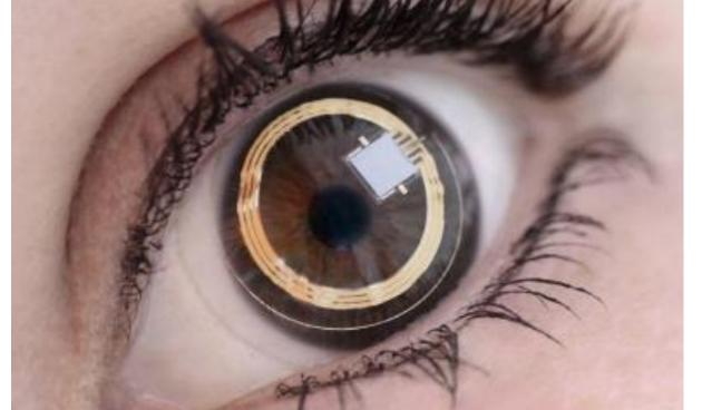
A Prototype Augmented Reality contact lens by Samsung
